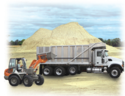
A front-end loader fills a dump truck with gypsum.
