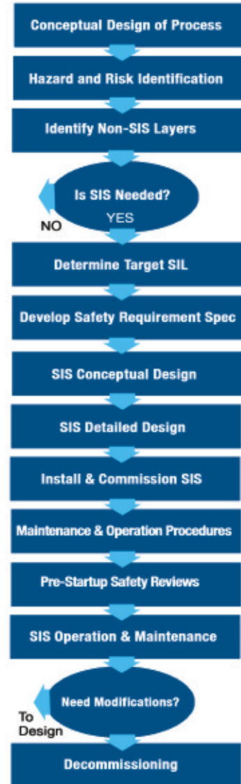
Figure D The Safety Life Cycle is a sequential approach to developing a Safety Instrumented System (SIS). References to a Safety Life Cycle can be found in ANSI/ISA 84.00.01 Parts 1–3; IEC 61508 Part 1; and IEC 61511 Parts 1–3.
