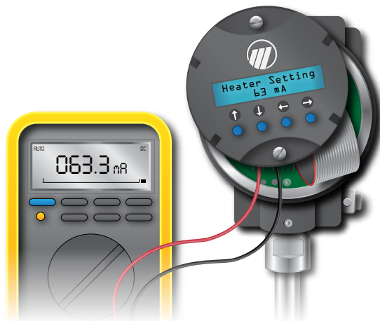
Test the Heater Setting Using a Multimeter
